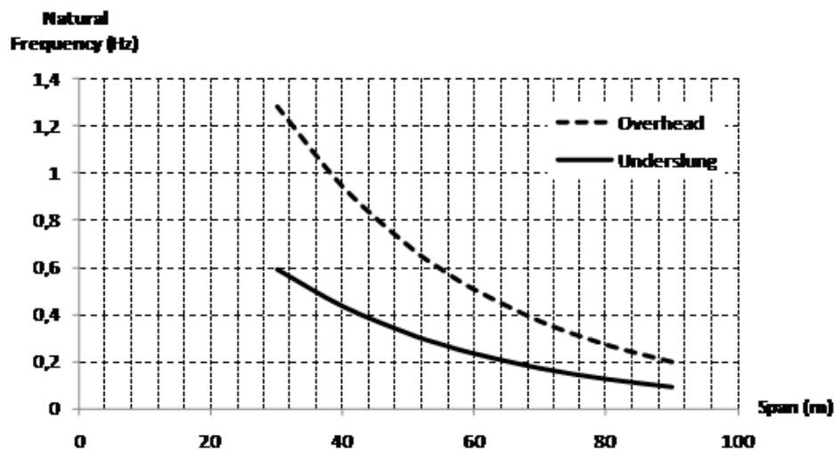
Figure 5: Natural frequencies on MSS (horizontal transversal mode) on maximum cantilever position during launching
