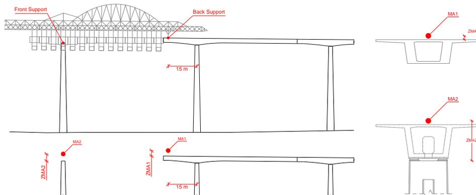
Figure 7: Location of LMSS plus liquid concrete mass in Rio Cabriel Bridge during concrete pouring operation
