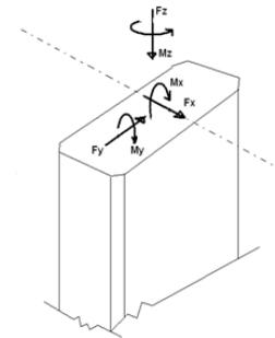
Figure 6: Service loads on the front pier in Rio Cabriel Bridge
