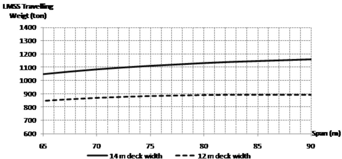
Figure 4: Indicative limits of LMSS travelling weights neutral for deck design
