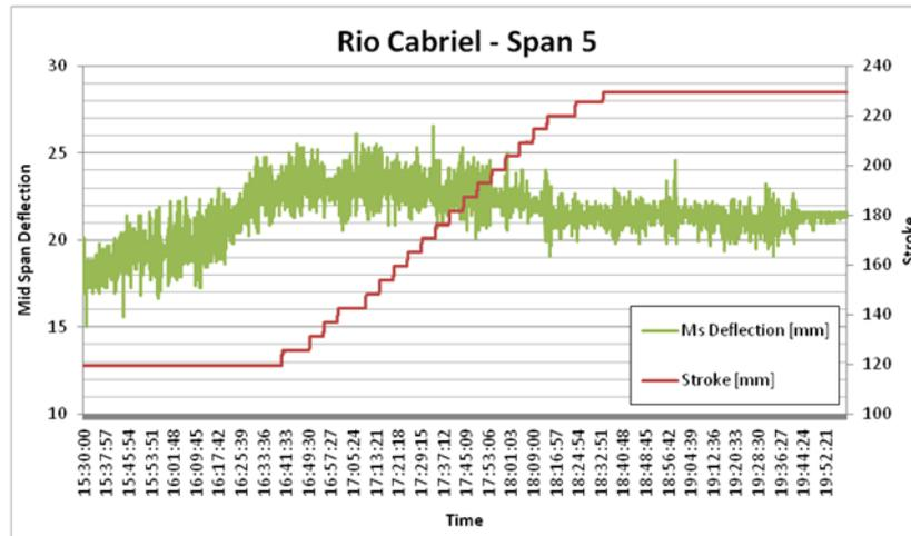
Figure 9: Measures of mid-span deflection and OPS actuators stroke during a concrete pouring operation in Rio Cabriel Bridge
